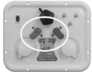
Fig 2: Set 2 Valves to 45°
