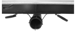
Black/Grey Tank Drain and Valves
